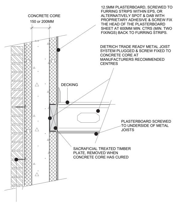
EXTERNAL FINISH INDICATIVE ONLY, HOWEVER IF USING BRICKWORK, BRICKS TO BE TIED AT 450mm VERTICAL CTRS & 750MM HORIZONTAL CTRS (NOT STAGGERED) USING STAINLESS STEEL WALL TIES SCREWED BACK TO FURRING STRIPS WITHIN EPS. LENGTH OF TIE TO SUIT WIDTH OF BRICKWORK
