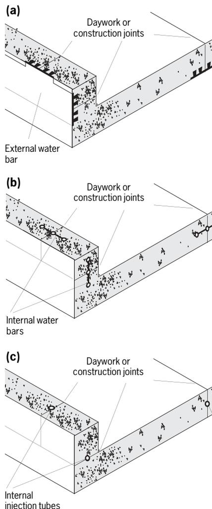
**Figure 4** (a) Dovetail section rubber or plastics strip cast into the shuttered face of the pour. (b) Dumb-bell section rubber or plastics strip cast into the open face of the shuttering. (c) Perforated tube cast into the open face of the pour for later injection of resins into the joint
