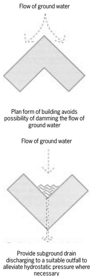
**Figure 2** Effect of building orientation on flow of ground water. Reproduced from *Approved Document: Basements for dwellings* by permission of TBIC
