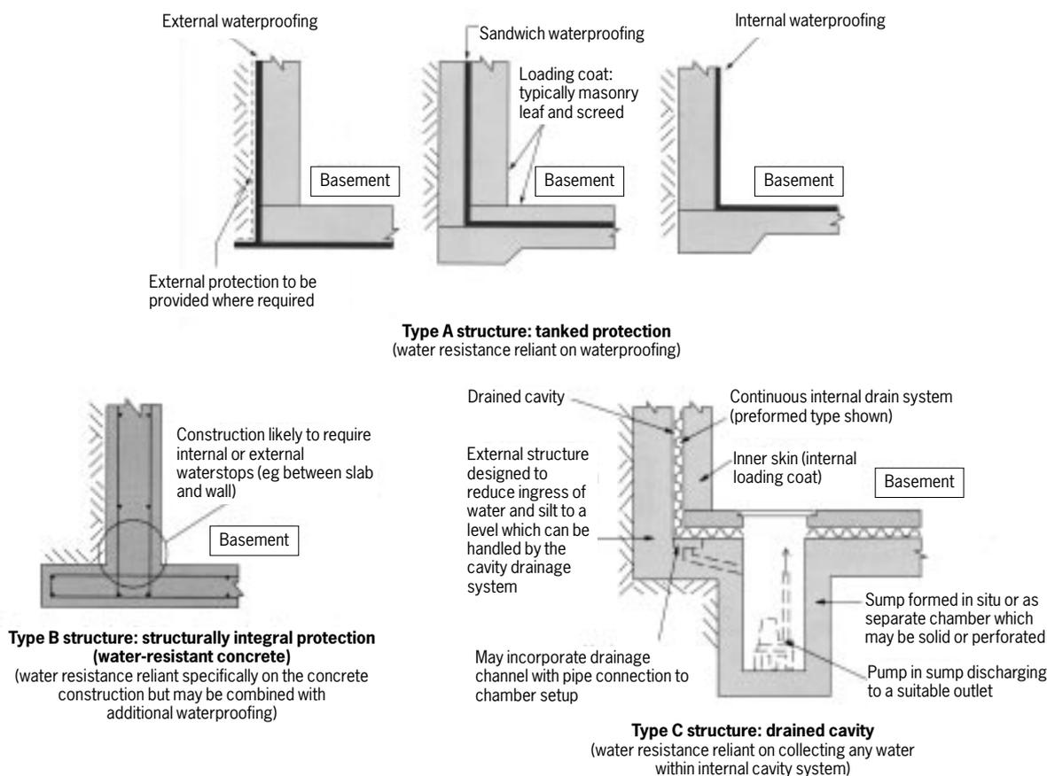
**Figure 3** The three types of basement construction. Reproduced from *Approved Document: Basements for dwellings* by permission of TBIC
