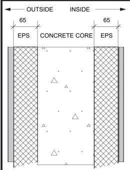
For either 150 or 200mm concrete core
